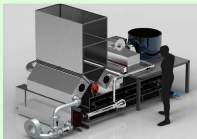
Fig. 3: Conceptual model of an industrial biochar pyrolysis unit in Switzerland. This minimizes the introduction of oxygen into the burning chamber and allows syngas, a by-product of pyrolysis, to be utilized as a source of heat and electricity as an alternative to fossil fuels (3).
